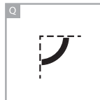
Q = 1/4 Cut out for inside corner
